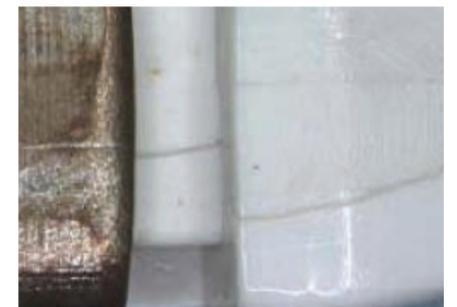
The white plastic tip of a linear cutter has become separated slightly, exhibiting a crack and blood and body fluid residues.
